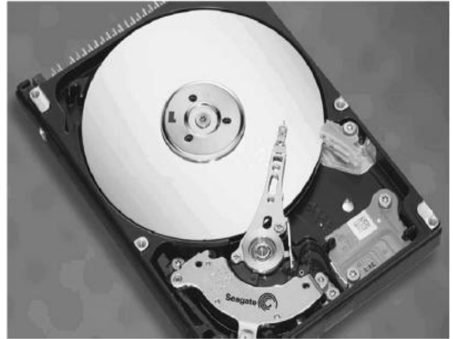
Fig. 1. Industry first 120 GB 2.5-in Seagate Momentus II high capacity mobile drive using TMR reading element.
